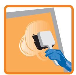
Apply XHR-AN using a brush to both sides of a screen. Leave about a 10" gap from the edge of the frame.
