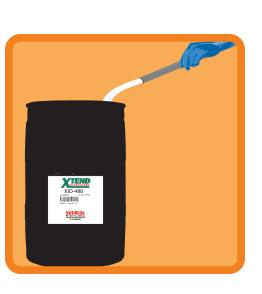
Add 2 gallons of XSR-155 stencil remover to a drum of XID-480/25 ink degradent and then fill the remainder of the drum with water.
