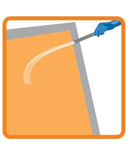
Apply XMP- Heavy Duty Mesh Prep to both sides of the screen and rinse off with a garden hose.
