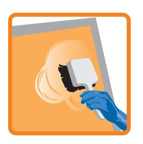
Apply XID-480 solution using a brush or spray to both sides of a screen.
